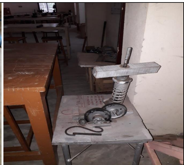
Manufacturing of Hump for Power Generation
